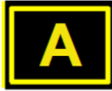
Taxiway Location Sign
