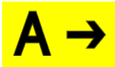
Direction/Runway Exit Sign
