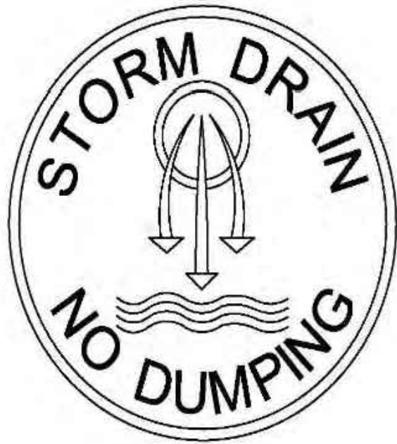
TYPE "A" TO BE INSTALLED IN WET CONCRETE DURING CONSTRUCTION
