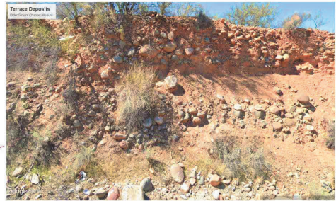
Picture 1 Coarse-grained Terrace Deposit Similar materials may be encountered within the alluvial profile above the Basin-Fill Deposits
