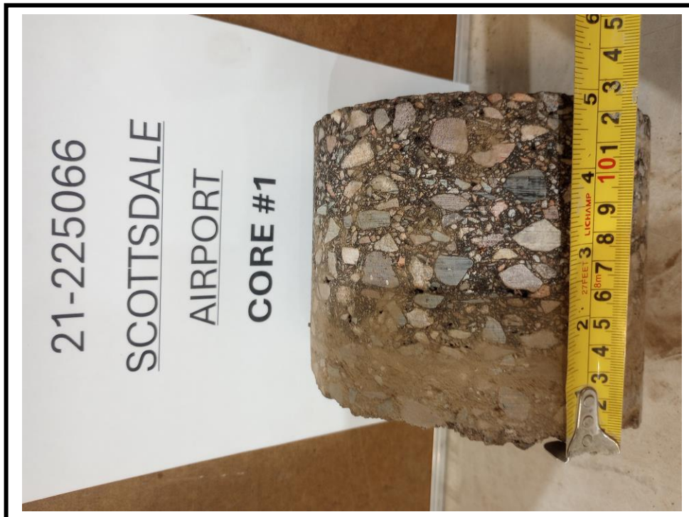
Picture No. 2 – Core No. 1, side view. 5" total thickness, 2.75" top layer.
