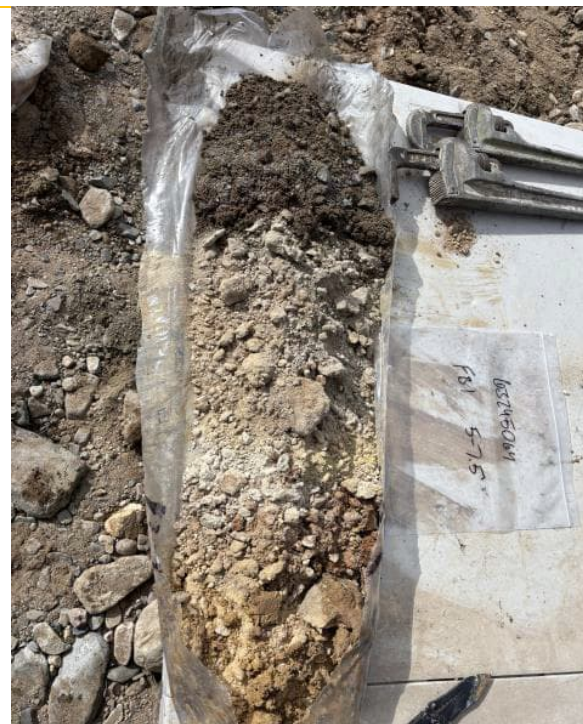
Continuous Sample for FB1 at 5 to 7.5 feet
